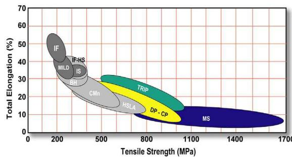
Figure 1: High Strength Steels (In Color) Compared to Low and Medium Steels (Dark and Light Grey)
