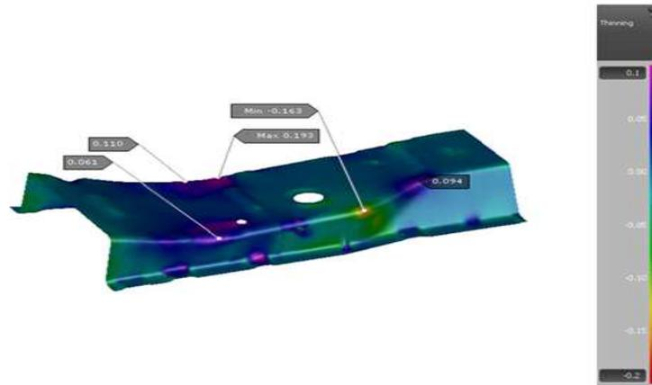
**Figure 6: Percentage Thickness Reductions for DP600 Material (Modified Design)**
